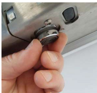
5. Fit the new aerator. MAKE SURE the rubber washer is in place between the aerator and the tap body.
