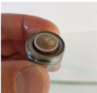
4. A new aerator and housing
