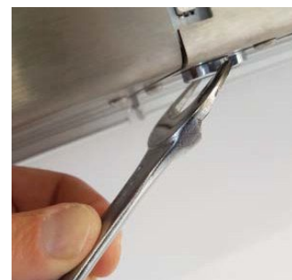
6. Tighten with a ½ turn – DON'T overtighten as the housing material is acetal plastic and easily stripped.
