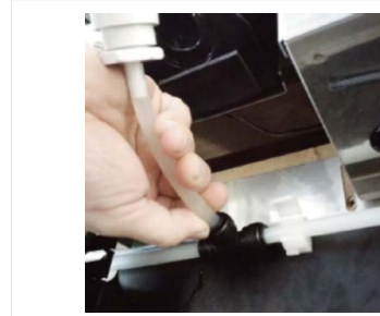
5. Disconnect pump from tee
