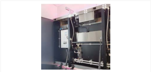
1. Open the left hand mirror to access the control box
