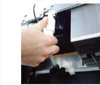
4. Remove pump from gearbox
