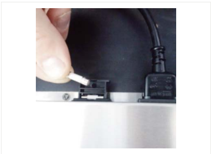
6. Replace the fuse in the holder
