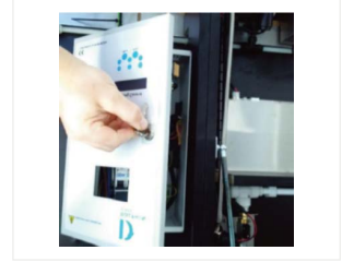
4. Open control box with the key
