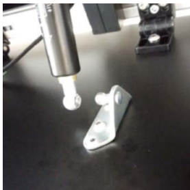
4. Pop top of strut off the bracket
