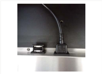
1. Slide open the fuse holder
