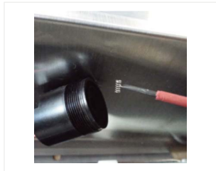
6. Remove the spring
