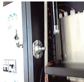
5. Pop bottom of strut off the bracket
