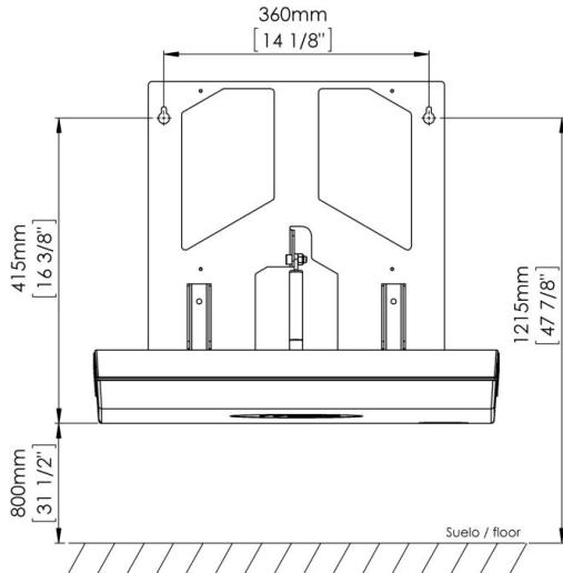
Following the above scheme, using the pencil, mark on the wall the top two holes of the changing station's holding structure. It is very important to make sure that the locations marked with the pencil for the mounting holes are at the same level before drilling the holes.
