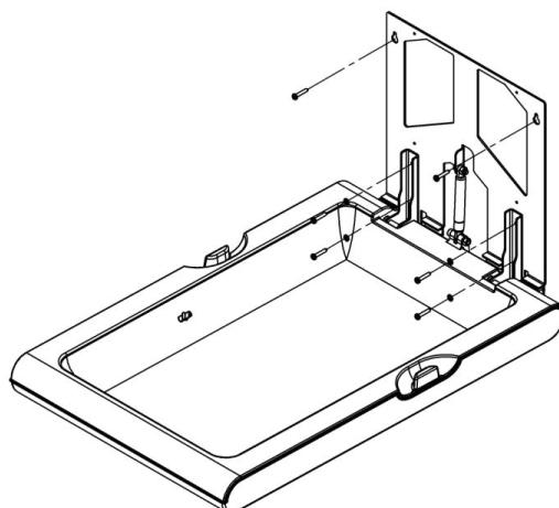
Make sure that the six screws securing the unit to the wall have been properly tightened and that the changing station is firmly fixed to the wall.
