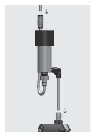
**IMPORTANT**: Make sure to cut the soap tube to the minimum required length
