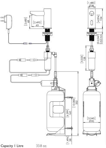
**Power Supply** 12V transformer Soap viscosity up to 100 cPs
